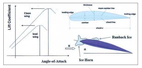
FIG. 2: The effect ice accretion has on the coefficient of 11ft and sta111ng angle-of-attack for a typical airfoil. Also sketched is an airfoil with leading-edge ice homs and runback ice (slightly exaggerated for better visual effects).
