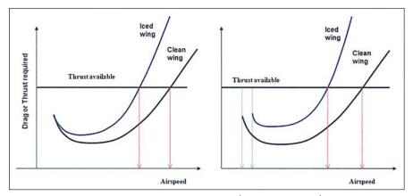
FIG.1 The effect ice accretion has on airplane drag (or thrust required) due to increase in parasitic drag only (left side). Increased weight and decreased coefficient-of-lift will result in even more inferior drag curve with accompanied higher stalling speed and slower maximum airspeeds (right diagram).
