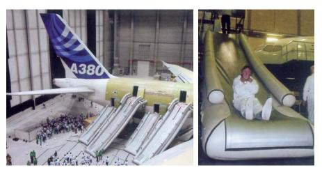
Above: an A380 has been cleared of 880 people in 74 seconds in test conditions Above Right: on the escape slides, it's important to hit the ground running
